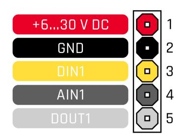
Figure 2 FMB920 pinout
