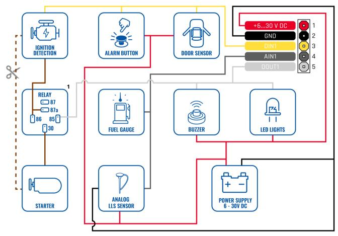
Figure 3 FMB920 Wiring scheme
