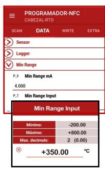
It automatically goes to the DATA tab, where we will see the parameters and we can modify them, accessing the drop-down menus (no longer having the mobile near the equipment).
