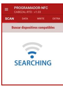
The SCAN tab allows you to read data already recorded in the equipment. By placing the device in contact with the mobile, the latter will automatically recognize the model. The APP emits a notification sound as soon as it detects the equipment and its parameters.
