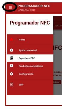
In the upper left part we find 3 small lines where we can access the configuration of the APP, see the equipment compatible with it, access help, exit and something very interesting: generate a PDF file with the configuration values of the equipment.
