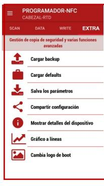
In the EXTRA tab we can access additional features such as saving or loading a configuration on the mobile, sending it by email or sharing it by whatsapp. We also have the possibility to restore the factory settings of the equipment.
