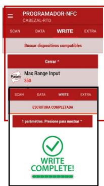
To load the new configuration into the device, we must access the WRITE tab where we will see the parameters that we have modified. This is where we will again place the mobile in contact with the device until we hear the notification that the operation has been completed.
