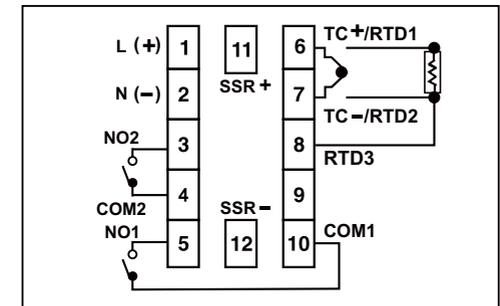
Use only the correct thermocouple wire or compensating cable from the probe to instrument terminals avoiding joints in the cable if possible. Failure to use the correct wire type will lead to inaccurate readings. Ensure that the input sensor connected at the terminals and the input type set in the temperature controller configuration are the same.
