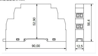
The equipment must be mounted on a DIN rail style DIN EN50022 inside a plastic or metal enclosure with a protection level >= IP65. All wiring must be secured. Maximum cable sizes 2.5 mm<sup>2</sup>. Connection clamp terminals.
