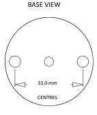
Mounting holes: two holes 5.5 mm diameter, 33 mm centres. Centre hole sensor wire entry 4 mm.
