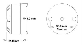
Mounting holes: two holes 5.5 mm diameter, 33 mm centres.
