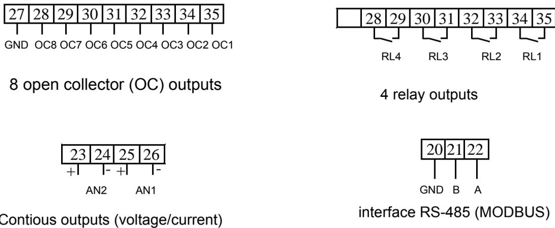
**Fig. 5: Output signals connection method**
