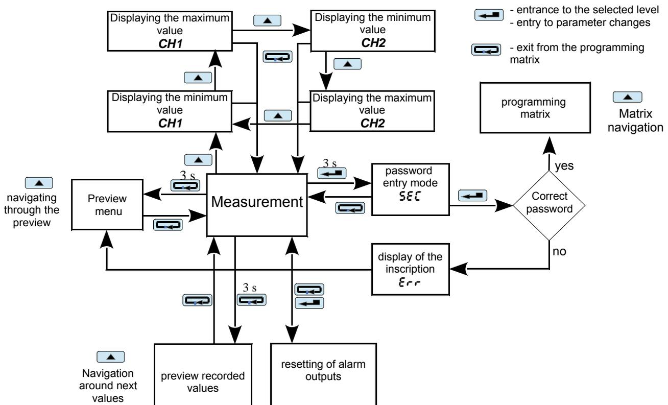
**Rys. 7 The NA6Plus meter operation algorithm**
