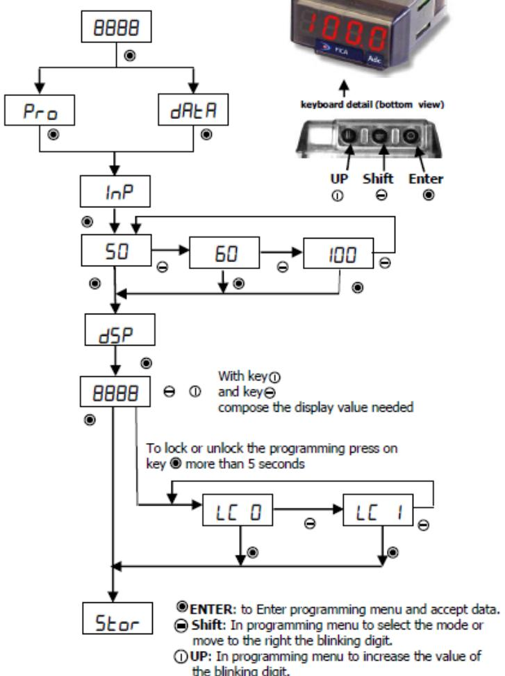
**InP:** Programming of shunt type used. 50 mV, 60 mV or 100 mV
